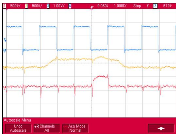
Fig. 6. Signals at three different stages showing the function of the multiplexing algorithm. Input address change from DAQ (top), output of stage 3 (center) and output of stage 4 (bottom).
